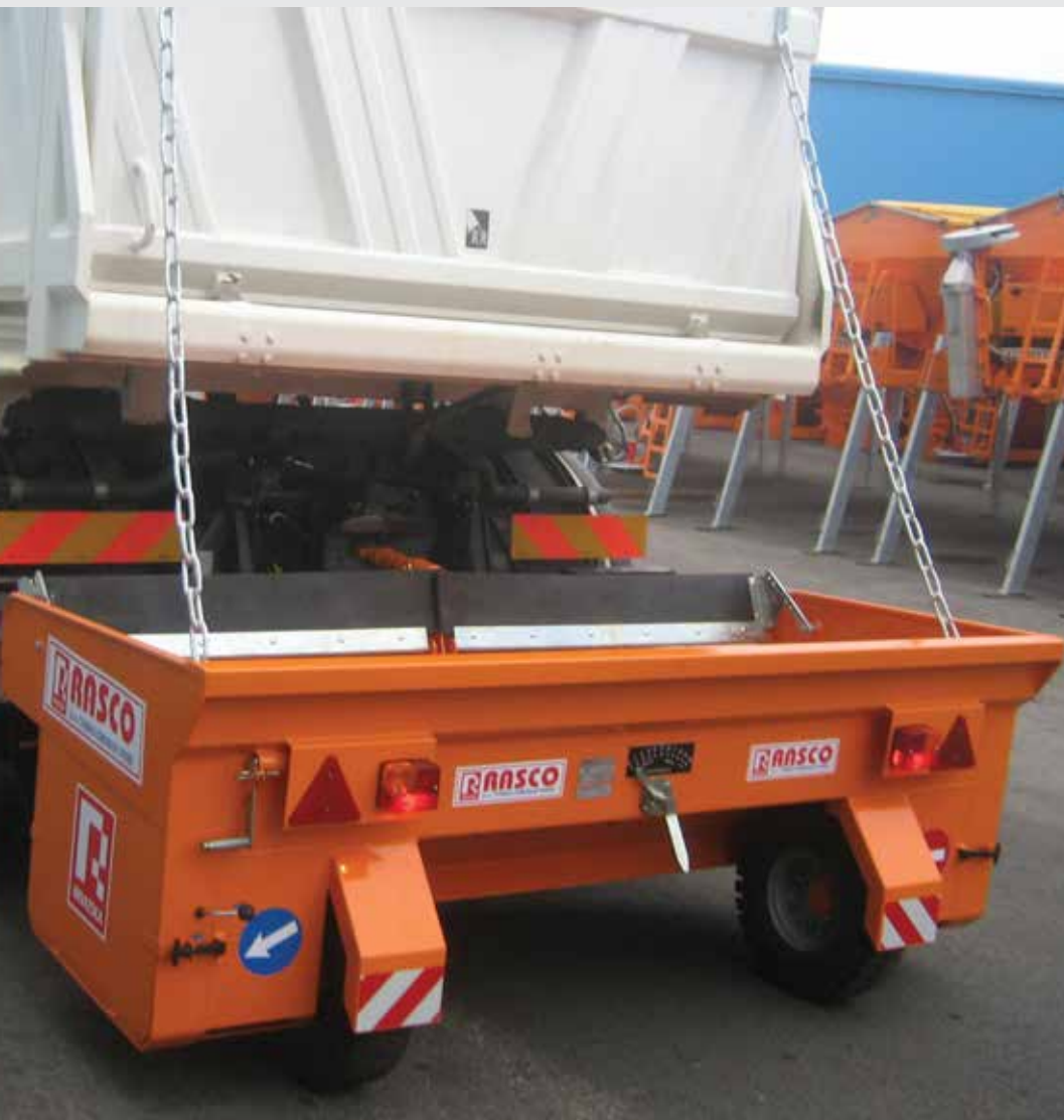
towed spreader RAS
