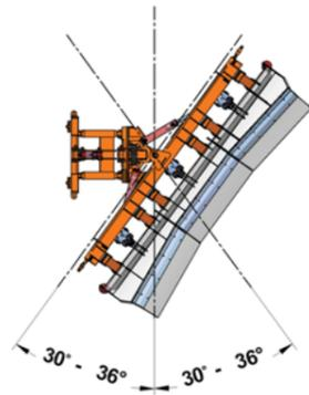
MOSOR PK snow ploughs are delivered with yoke which allows change of snow clearance angle between 30° and 36°, depending on need and type of snow. Wider angle is usually used for wet and heavy snow.
